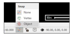
In using any of the snapping tools sometimes you might find that you are unable to locate a point to snap to on your surface and in this case it means your snapping depth is set too low. To fix this go to **Scene Properties**, **Editing** tab, and by **Snapping depth** you can change this to a higher amount:
