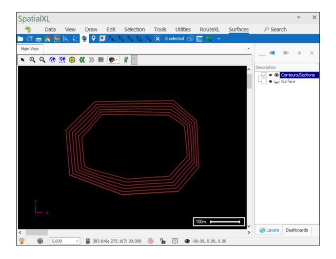
If you want to make closed polygons between levels instead of contours then make sure to have **Make closed polygons** ticked on before contouring:
