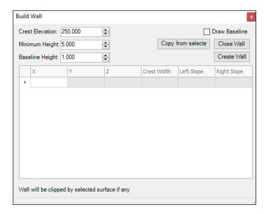
**Crest Elevation** is the height of the top of your wall in meters:
