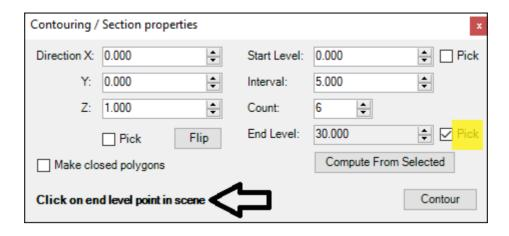
Clicking on the **Compute From Selected** button will compute start and end levels from the selected surface (if the parameters you have entered in make sense, then nothing will change):
