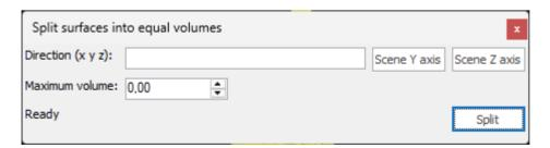
The Direction (x y z) field can be specified manually, or you can get the Y or Z axis of your scene by clicking the "Scene Y axis" or "Scene Z axis" button.
