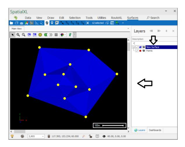
Your surface has been created and you can then turn off the points layer and rotate the surface to see it clearly. To rotate a surface or any 3D object simply choose one of the **Snap** tools by clicking here at the bottom of the spatial pane:
