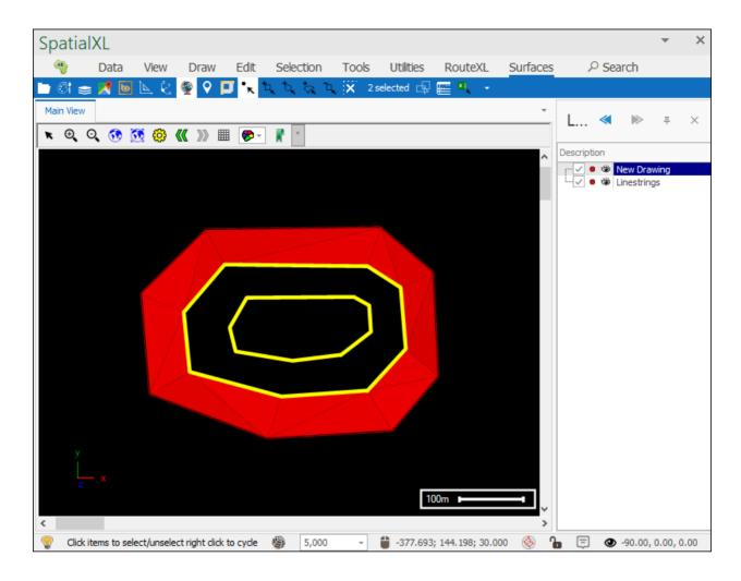
And click the **Build surface between closed strings** tool to build the next surface:
