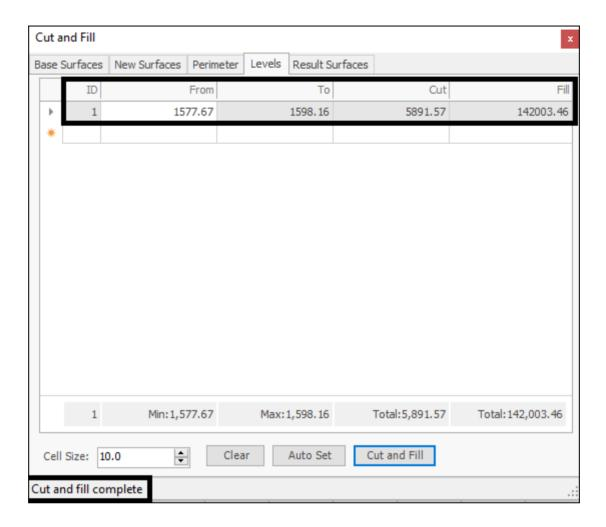
The elevations **From** and **To** are populated together with the square meters for the **Cut** and **Fill**.
