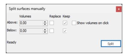
The surface will be split horizontally across the fixed Y axis of the screen as you look at it, so you can rotate the scene in the desired orientation, and it will still split the surface accordingly. The "Above" field will show what the volume of the higher (vertically as you look at the screen straight) section of the surface split will be and the "Below" field will show the volume of the lower section of the split.
