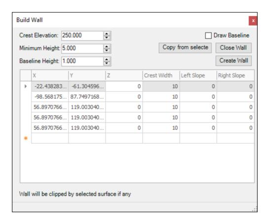
And you can now set the **Crest Width**, **Left Slope** and **Right Slope** (the slopes are expressed in units of horizontal distance divided by height, so if you have a 4 meter high wall and choose 1 meter horizontal distance then this would be 1/4 = 0.25 as your slope; smaller numbers means a steeper slope, bigger numbers will give you a more gradual slope):
