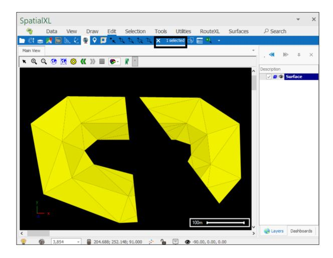
Then select the **Explode to connected** tool and the components will have been separated into two different surfaces:
