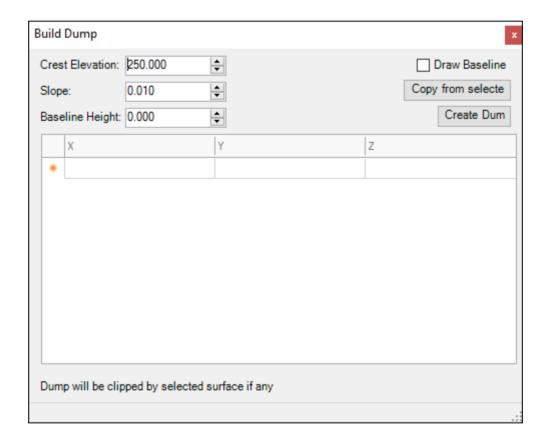
**Crest Elevation** is the height of the top of your dump in meters:
