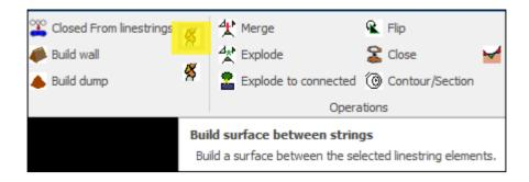
This tool allows you to build a surface between a pair of linestrings.
