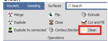
The "Clean" tool can be used to clean up a surface of small artefacts/parts and repair it as needed.
