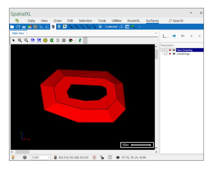
These last two tools are useful for creating surfaces where if you just used the **From linestrings** tool the surface might not be created so accurately. Here you can step by step create each part of the surface by only making a surface between two closed linestrings at a time.
