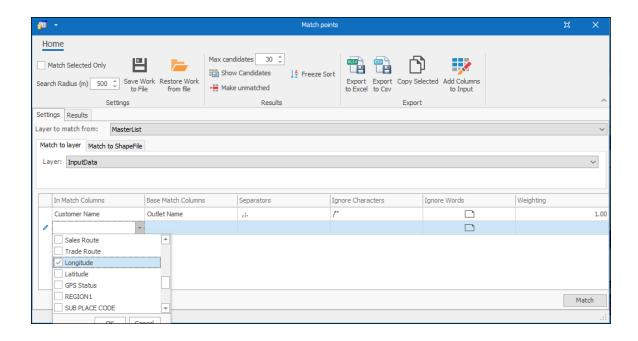
In the ribbon of the Match Point Tool you will see you can specify the **Search Radius** which basically tells the tool to search only within the given distance for matches. And you can also specify **Max Candidates** which will tell the tool what is the limit on how many matches it can find for each point:
