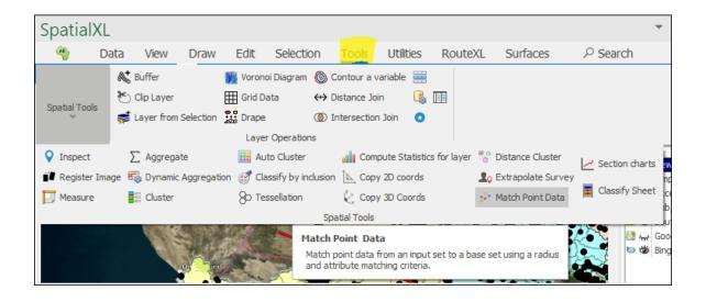
It is used when you have two sets of points which have the same points but maybe with slightly different coordinates or a different name for the point in each set; the sets would be from disparate sources. It is used to verify that your base set is correct and is not missing any points. It can then be used, once you've verified that the points in your base set are good, to do a gap analysis and see where you are falling short and who you are not reaching.
