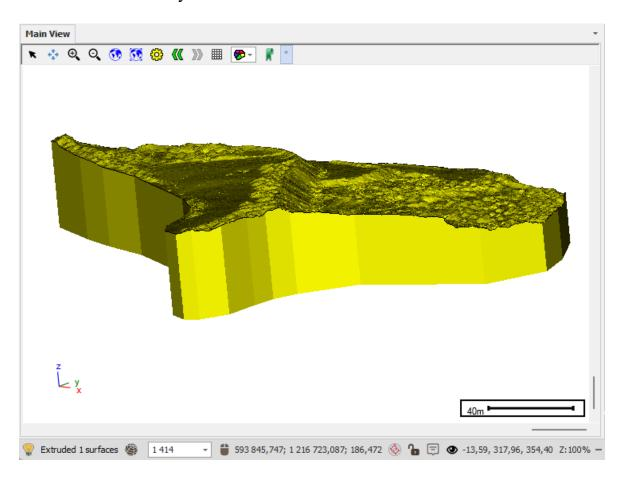
If we view the properties of the surface by clicking on the Inspector tool ?, and then click on the surface to select it, we can see that it is a proper closed surface and we can see it's volume:
