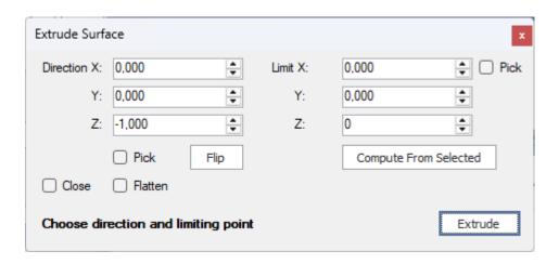
When you extrude a surface, it will choose a direction to extrude it in, the default it gives you is Z: -1 which is in a downwards direction.
